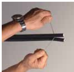
The picture shows the necessary operation to split the twin hose.
